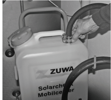
2. Connect return hose to tank.
